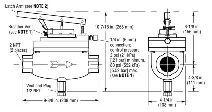
**NOTE 1:** Control pressure connection fitting and breather vent fitting can be swapped to convert to vacuum control. **NOTE 2:** Thumb operated opening latch (2.5 psi [17 kPa] [.17 bar] required to release cocking latch).
